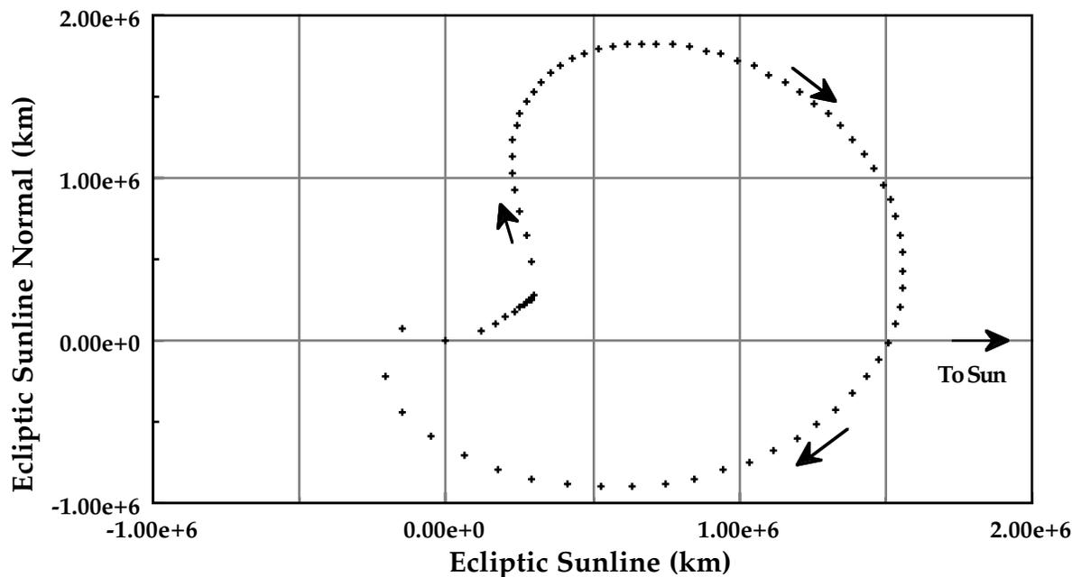
**Fig. 5 Angular Momentum Reversal Phase of the Triple Lunar Swingby**
